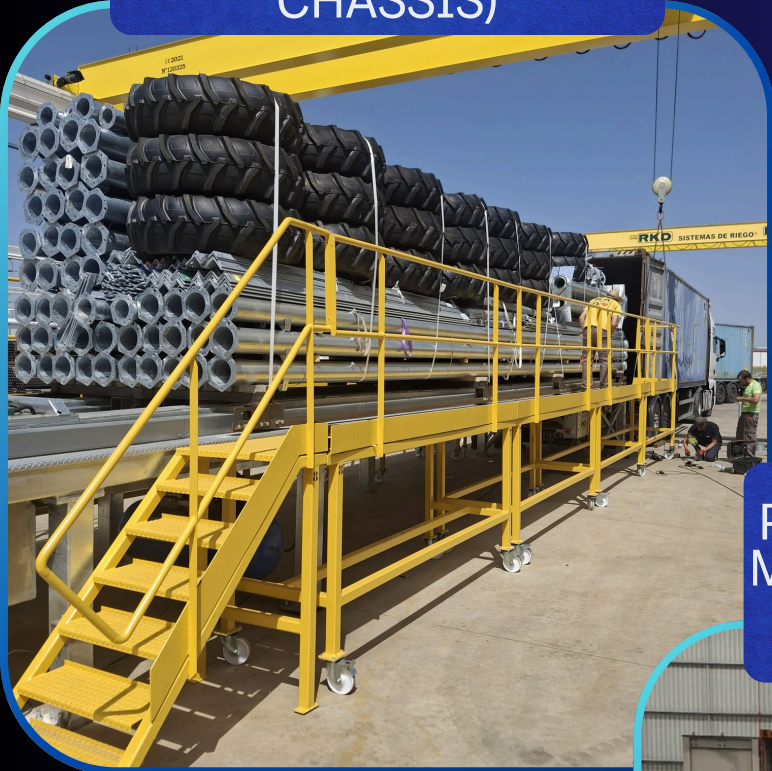
FIXED PLATFORM (LOADING AND UNLOADING ON TRUCK CHASSIS)
